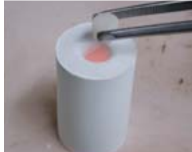
Insertion of the Ingots
