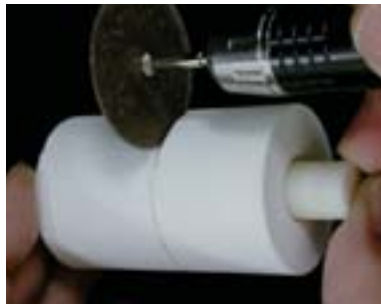
Section with a separating disk
