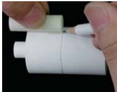
Marking the top position of the plunger
