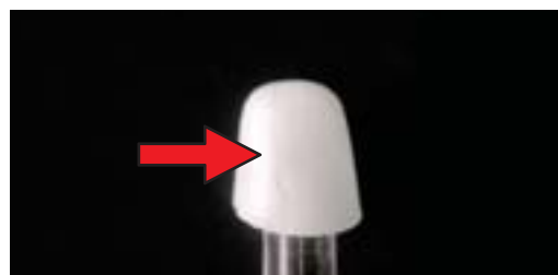
Crack is happened during grinding
