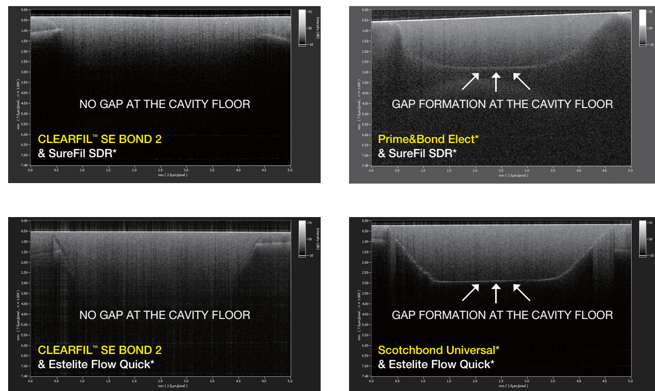
Fig.18 Optical Coherence Tomography (OCT) images of the bonding interface with composite.
