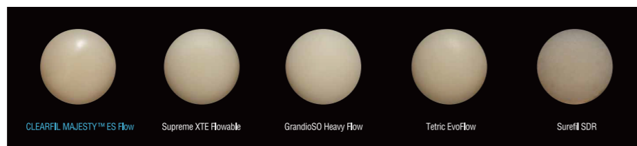
Fig.1 : GLOSS AFTER WIPING WITH ETHANOL
